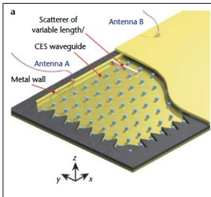
(a) A model of the photonic crystal. The distance between the ferrite rods is 4 cm.
