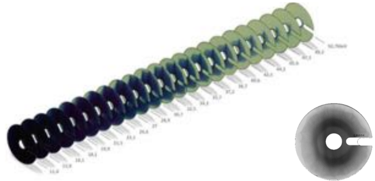
Radiochromic film images (EBT3) due to protons obtained in shot #176: 450J/610 fs on a 50 \mu\text{m} thick plastic target (CH+1 \mu\text{m} Al). Right: annular distribution pattern on HDV2 radiochromic film (protons around 9 MeV)
